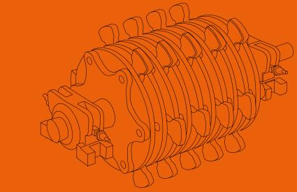
Up to 1500 HP, **LEFORT** • hammermill shredders can process a wide variety of ferrous and nonferrous materials such as light scrap, end-of-life vehicles or household appliances.
